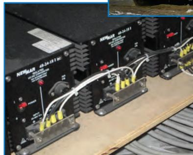
Isolated converters in parallel/redundant configuration deliver noise-free and regulated voltage to propulsion system controllers.
