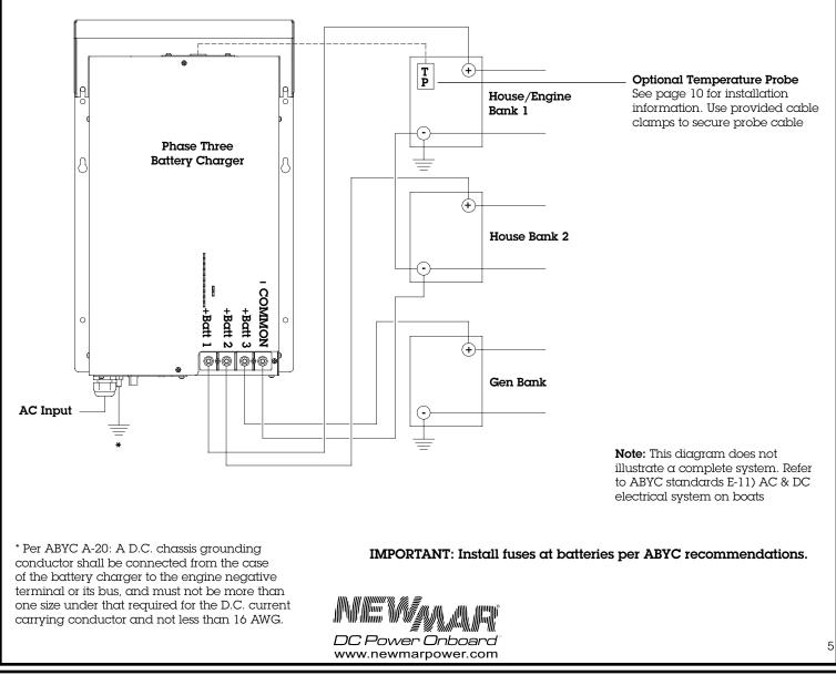
FIGURE 1: Simple D.C. Wiring (Preferred Method)
