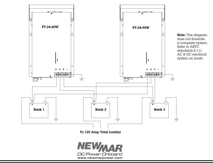
FIGURE 4: Parallel Wiring for Large Capacity Battery Systems
