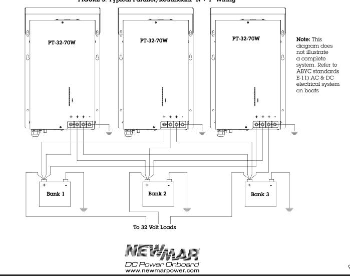
FIGURE 5: Typical Parallel/Redundant "N + 1" Wiring
