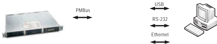
Figure 3 Diagram of the communication interface of the Scout-S
